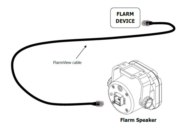
If the flarm can not provide 12volts, the following diagram represents how Flarm Speaker should be connected.
