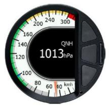
QNH display will be automatically closed a few seconds after the last button was pressed.
