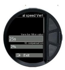
TE compensation is used mainly for gliders in order to show total energy change rather than vertical speed. Set to 100%, if you want to have compensated vertical speed indication or leave on 0 to have non-compensated vertical speed.
