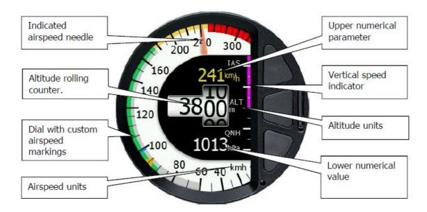
In the middle of screen, altitude is displayed as rolling counter. On the right side vertical speed is drawn as a magenta bar. Additionally, two numerical values can be shown. See chapter 5.3.1 on how to customize main screen.
