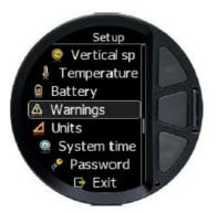
When you press the middle button for a longer time, you will get into the setup menu. Press the upper and lower buttons to move focus. Quickly press the middle button to enter the submenu. Long press the middle button to exit the submenu or select the Exit option in the menu.
