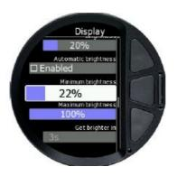
Press the middle button to enter edit mode. The slider background color will change to white. Use the upper and lower buttons to increase or decrease the value. Long press will make a bigger increase or decrease. Confirm selection with a short press on the middle button. Long press the middle button to cancel selection and exit without changes.
