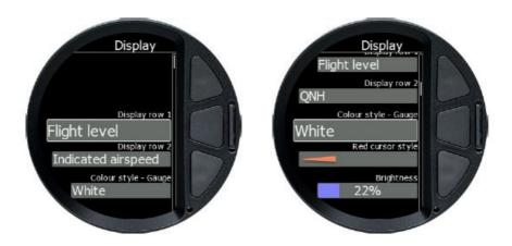
**Display row 1 and Display row 2** are used to select values that are shown in top row or bottom row. User can select among the following options: QNH, Battery voltage, Outside temperature, Vertical speed, Density altitude, Flight level, Height above take-off elevation, Altitude, True airspeed, Indicated airspeed and none. Color style – Gauge defines the background color of the airspeed dial, which can be black or default white.
