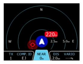
Targets are displayed as a series of symbols, as shown in the table below. It's also possible to change the object colour, depending on the relative altitude to the airplane. You can do this by going to Setup-> Graphic-> Traffic. All received targets (Flarm or PCAS) are marked with the same type of symbol except undirected targets, for which we don't know what direction they are travelling to. Flarm targets can be separated only by their ID.
