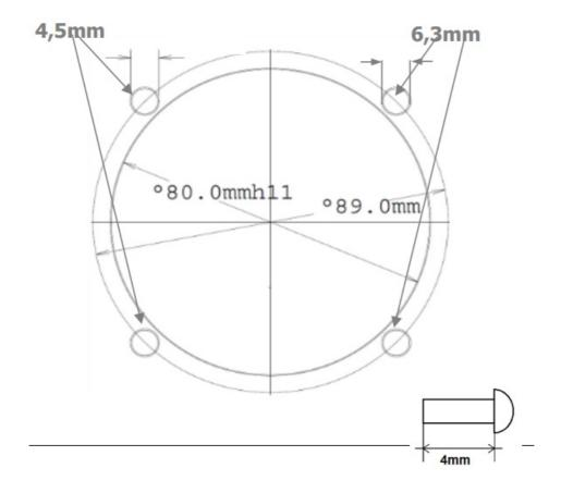
The length of the M4 screws is limited to 4mm!!!!
