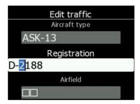
Pressing the right push button will move the cursor right. The left push button will move the cursor left. At the last character position, the right push button will confirm the edited value, a long press to the rotary push button will cancel editing and exit that control. Middle push button will delete selected character.
