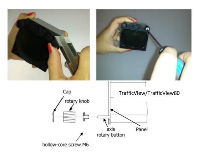
Remove the two rotary knob caps with a knife or a flat screwdriver, then hold each knob and unscrew it. Remove the remaining two screws and the two M6 threaded nuts. Install the knobs and the panel there is sufficient space so that the button can be pushed.
