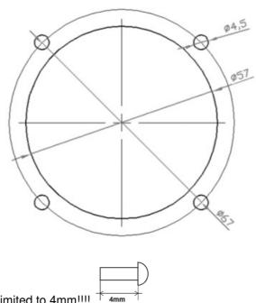
The length of the M4 screws is limited to 4mm!!!! 1 4mm
