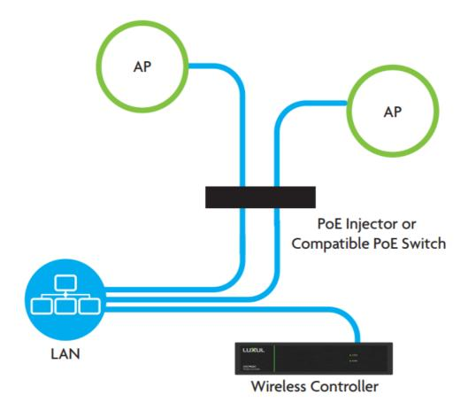
Connecting Devices: The XWC-1000 Wireless Controller simply connects to the network along with any compatible Access Points.
