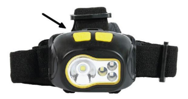
**Flood On/Off & Cycle Modes:** Press and release the button on the left of the headlamp to turn flood light on. Press button repeatedly to cycle through modes (White/Green/Red).
