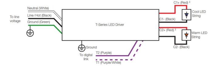
‡C1+ and C2+ are electrically connected inside the driver. This supports the use of common anode loads.
