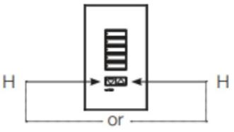
4. Press and hold Open for 5 seconds to store the open limit or Close for 5 seconds to store the close limit
