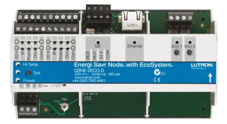
Buttons and LEDs in the module are used for programming and troubleshooting. If wiring is exposed when accessing buttons and LEDs, the module must be accessed by a certified electrician, following local codes
