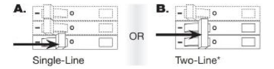
• Wiring must comply with NEC code for wiring Multiple Branch Circuits: Where two or more branch circuits supply devices or equipment on the same yoke, a means to simultaneously disconnect the ungrounded conductors supplying those devices shall be provided at the point at which the branch circuits originate.
