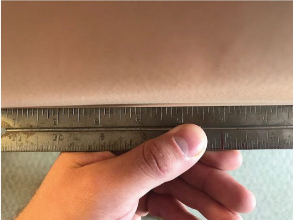
Photo of straight edge used to evaluate wall flatness.
