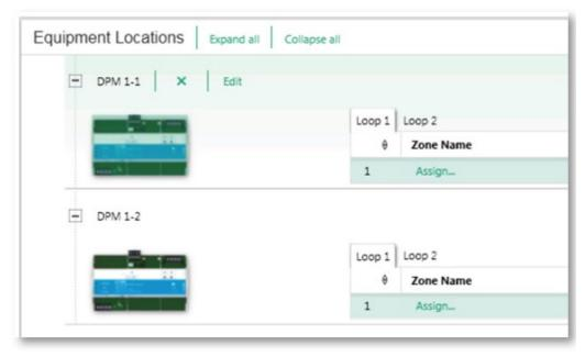
3. Click on the Assign link in the Zone Name field for the Power Module that will have drivers/ballasts assigned to it. Assign each driver/ballast to the appropriate EcoSystem link and address (1 – 64). See below for an example of drivers/ballasts assigned to EcoSystem link 1. Notice how the Load # of each driver/ballast clearly defines the Panel #, Power Module #, EcoSystem link #, and address.
