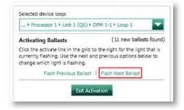
**Example:** Drivers/ballasts are being activated in the Great Room. Click Flash Next Driver / Ballast until a fixture in the Great Room begins to flash. Using the ceiling plan with the load numbers of each EcoSystem fixture, identify the fixture that is flashing and click Activate in the Action column for that fixture.
