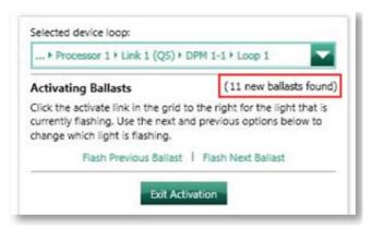
5. Click Customize columns and click the box Show only unactivated drivers/ballasts. Notice how the last number in each parentheses matches Address On Link. This will help in the addressing and troubleshooting process.
