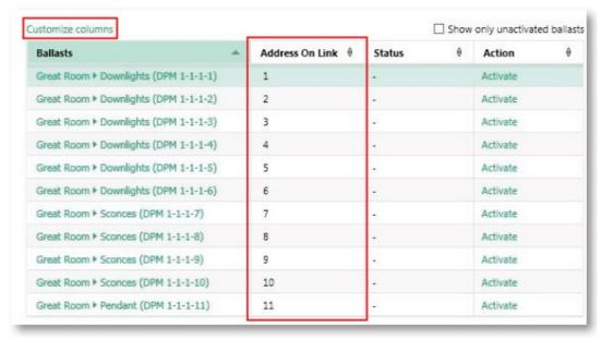
6. A random fixture on the link will begin to flash in order to identify itself. If there are multiple areas on the same EcoSystem link (which is likely), it is easiest to address drivers/ballasts on an area-by-area basis rather than walking throughout the residence trying to find the fixture that is flashing. To aid in this process, click Flash Next Driver / Ballast until a fixture in the area to be activated starts to flash.
