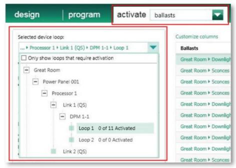
2. After selecting the EcoSystem link to be activated, verify the wiring of all drivers/ballasts on the link by clicking High End, Low-end, and Off. If any drivers/ballasts fail to respond as expected, correct the issue before proceeding.
