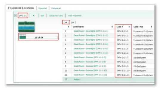
4. After assigning all EcoSystem drivers/ballasts to the appropriate EcoSystem links, assign all Power Module to the QS link of the processors on the design > Link Assignment screen. Remember that each Power Module counts as 1 of the available 99 devices on the QS link. Also, each zone of EcoSystem drivers/ballasts (not each driver/ballast individually) counts as 1 of the available 512 zones on the QS link.
