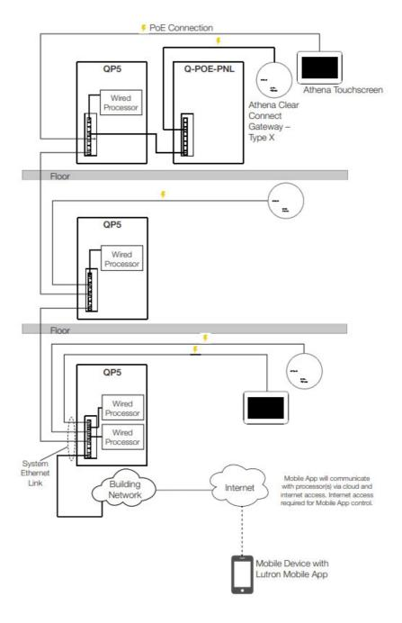
**Note:** Connecting all Athena processors, Clear Connect Gateways – Type X, touchscreens, and LTE modems via the system Ethernet link is required for startup and operation of the system.
