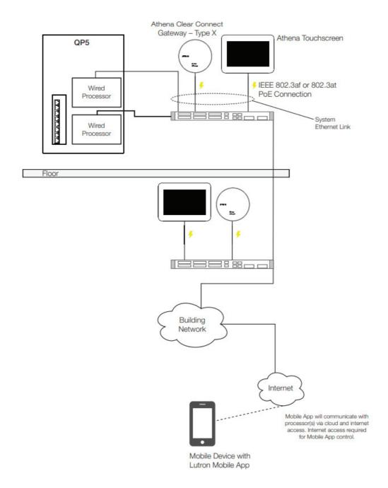
**Note:** Connecting all Athena processors, Clear Connect Gateways – Type X, touchscreens, and LTE modems via the System Ethernet Link is required for startup and operation of the system
