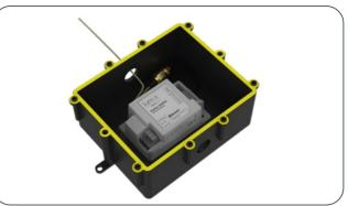
3. Take in the DALI wires from the driver through the connector on the box and connect them to the DALI push-in connectors on the device. Also, take out the wire antenna through the same connector
