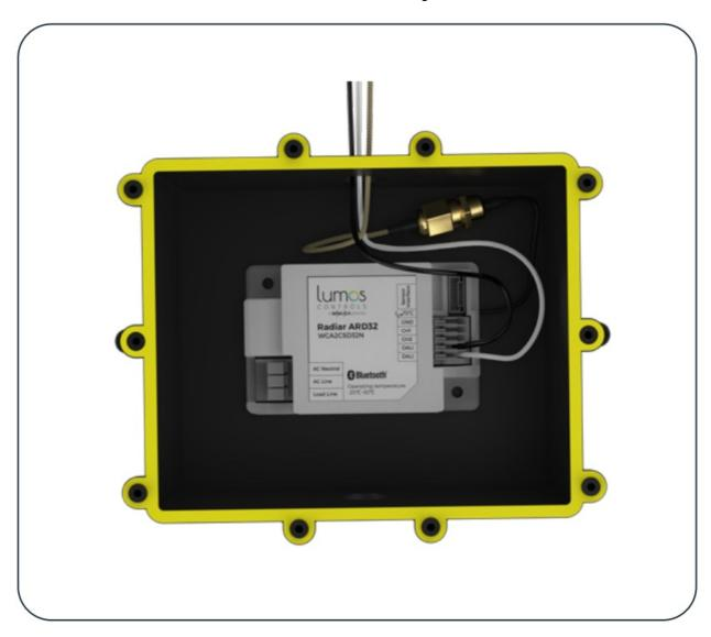
4. Take in the AC wires from the Mains through a connector (in the box) and connect to the AC Line(Brown) and AC Neutral(Blue) push-in connectors in the device.
