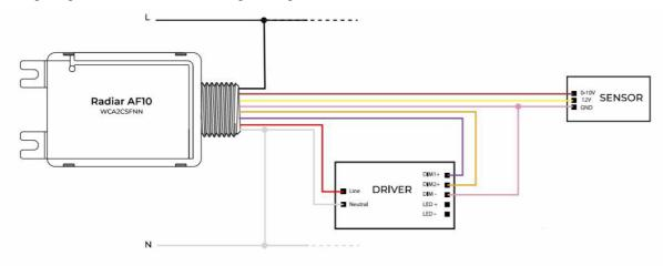
2. Configuring Radiar AFIO for dimming, tuning and an external sensor control (with additional surge protection)
