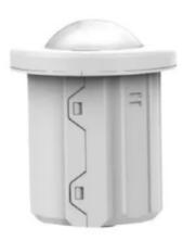
Cyrus AP is a BLE5.2 controllable high bay PIR motion and daylight sensor. This sensor operates on a 90-277VAC input voltage range adopts a PIR sensing technology for accurate motion detection. It comes with swappable lenses for high-bay and lowbay applications, giving you a maximum mounting height of 14m (46 ft) and a maximum detection range of 28m (92 ft) diameter.
