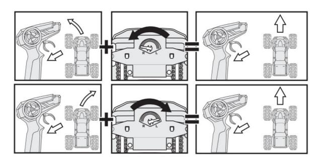
Under your LUMITEK RC™ TERROR TOWER is located a pin that you can turn in order to adjust the wheel alignment if you find out that your truck does not drive straight when not turning the wheel. Check the diagrams above to find out how to adjust on the right or on the left.
