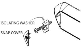
When predrilling mounting screw holes use an appropriately sized bit for the composition and thickness of the mounting surface. Most applications will require a drill bit sized larger than the minimum diameter of the screw, but smaller than the maximum thread diameter.
