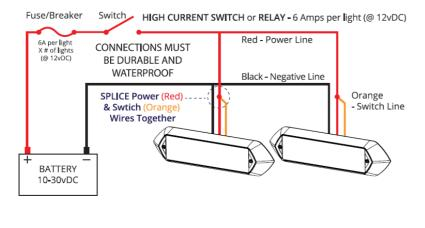
**NOTE:** The JAVELIN can also be wired in a standard two wire installation as well by simply connecting the red and orange wires together and powering via an appropriately rated switched power buss.
