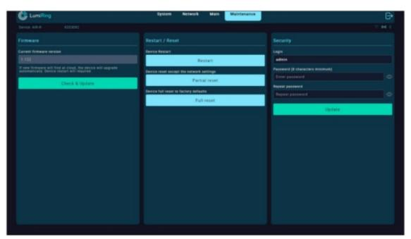
The Firmware section displays the current version of the unit's firmware.
