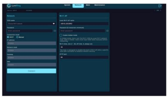
In the Network section, you can set up an Internet connection via Wi-Fi or Ethernet, you can change the connection settings for the built-in Wi-Fi AP, and you can set its activity time.
