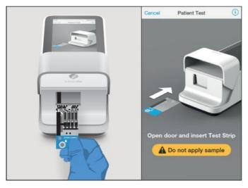
3. When prompted, open the Instrument door and gently insert the Test Strip as far as it will go. The thick black alignment rib on the Test Strip should be on the left and line up with the black line on the Instrument. Do not apply the sample until prompted. Install
