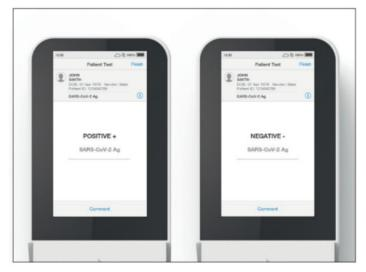
8. Results are displayed within 12 minutes of applying the sample. The left-hand image here shows a positive result for SARS-CoV-2 Ag and the right-hand image shows a negative result for SARS-CoV-2 Ag. Tap Finish to complete testing or tap Comment to leave a comment or to reject the Test, then follow prompts to return to the Home Screen. All test results must be read using the LumiraDx Instrument.
