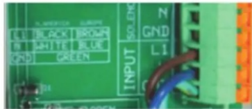
Figure 3 Wiring Colour Guide
