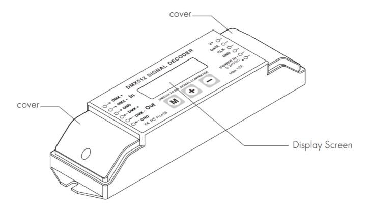
Prior to installing determine the location, which requires a minimum of 2" clearance around the decoder to provide proper air circulation.
