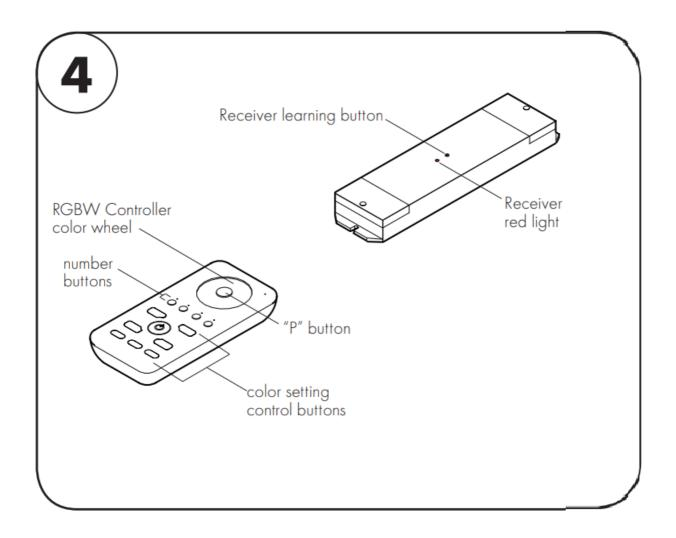
Every zone has to have a paired receiver to it before it can be assigned a color setting. Follow instructions on step 3 to pair receivers to any given zone (number on remote controller).
