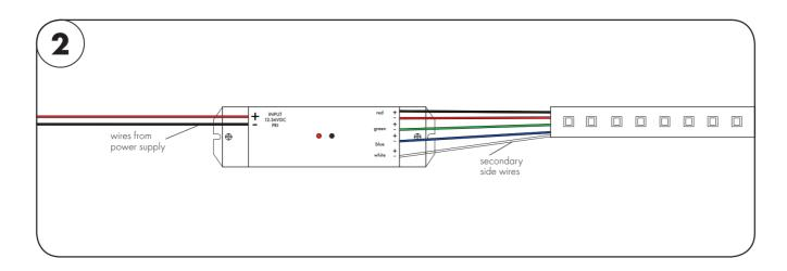
Connect the black negative wire from power supply to "-" minus sign on Receiver's primary side. Then connect the red positive wire from power supply to "+" plus sign on receiver's primary side.
