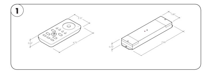
The RGBW controller can keep track of up to 4 different lighting zones (settings). Each zone can be associated with more than one receiver. Each receiver can memorize one static color and one sequence of colors at a time.
