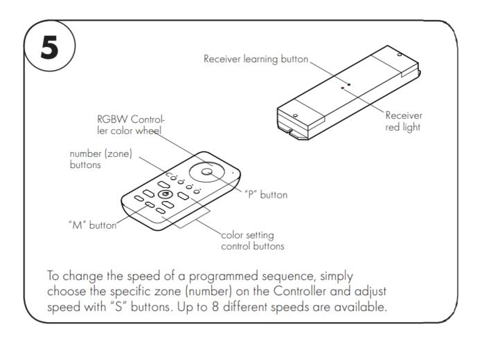
To change the speed of a programmed sequence, simply choose the specific zone (number) on the Controller and adjust speed with "S" buttons. Up to 8 different speeds are available.
