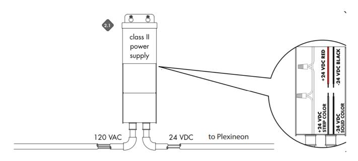
**2.1** Connect +24 VDC strip color from the Plexineon to the power supply +24 VDC red wire. Connect -24 VDC solid color wire from the Plexineon to power supply -24 VDC black wire.
