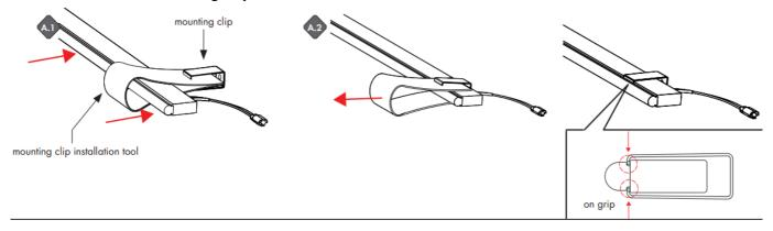
**A.1** Make an U shape with mounting clip installation tool, insert two edges into mounting clip. Place plexineon fixture insde the shape. Then push the fixture into clip.
