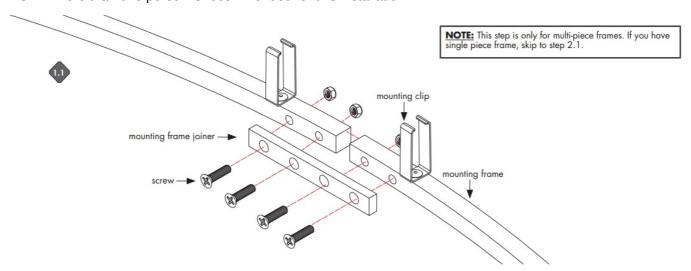
For multi-piece frames, connect the frame members together with mounting frame joiner. Use locknuts to secure connection.
