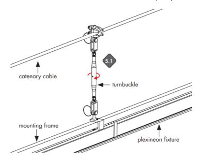
**5.1** After installing plexineon with catenary cable, adjust the length by rotating the middle part of turnbuckle. **NOTE:** Turnbuckle is adjustable up to 2.5" vertically.
