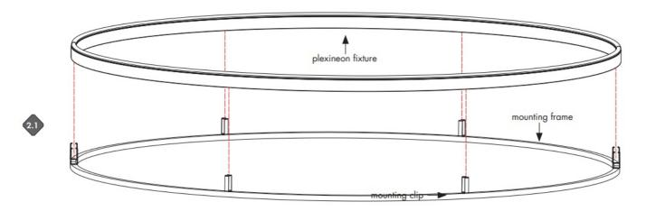
Install plexineon fixture to mounting clips on mounting frame(s).
