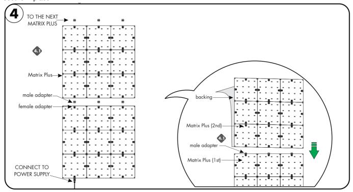
**OPTIONAL:** There are 2 additional mounting options, when the adhesive tape is not sticking on to the surface properly. The first and easier solution is to use push-pins (ii applicable). Only can be used in the areas on the board outlined with a push-pin illustration. The second is to use #0 screw size with an electrical insulating polypropylene plastic washer 0.065"ID, 0 .188" OD. Insert the screw/washer through the Matrix Plus mounting holes to secure Matrix properly to surface.
