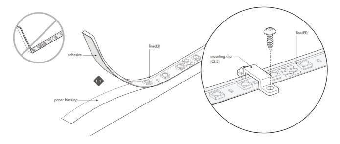
**NOTE:** Avoid bending the line in sharp horizontal angles, doing so can cause damage to the LEDs.
