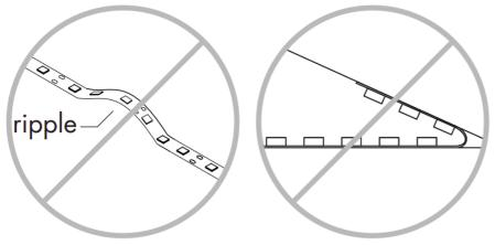
**NOTE** – Avoid sharp bends or bending near 1" on the solder joints.
