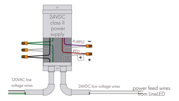
Connect positive middle wire (plus sign tag) to RED low voltage wirefrom power supply. Also, connect BOTH negative wires (no tags) to PURPLE low voltage wire from power supply
