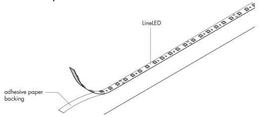
NOTE When removing backing & laying Line LED to surface avoid installing with ripples & bending over 90°.
