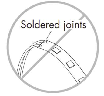
If length of Line LED needs to be adjusted on site, simply cut the LED strip in between solder pads. Always cut from end with no connector/wire leads.
