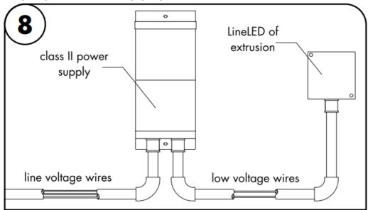
8.1 Ensure the correct (wattage & voltage) power supply is used to power LineLED.
