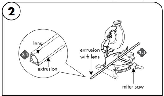
**Caution:** Safety equipment is recommended, when modifications are being made to the extrusion & lens. 2.1 If necessary extrusion, lens, & mounting channel (if applicable) can be cut in the field. Snap all parts together then using the proper blade for aluminum cut to the desired **length.**
