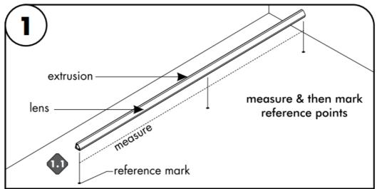
**Note:** Complete fixture must be built prior to installing. To make all necessary reference marks & to also ensure all parts are included. Then it can be taken apart for installation.
