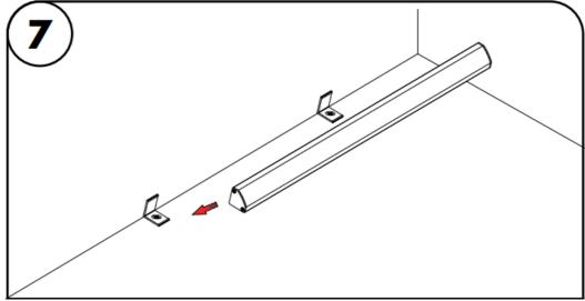
7.1 Snap the fixture into the installed mounting brackets.
