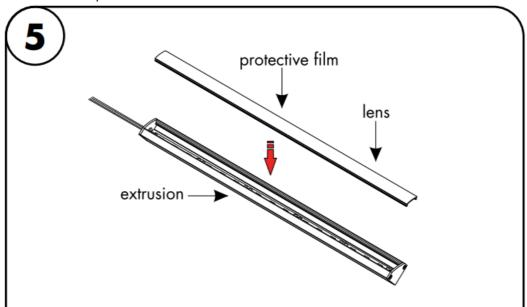
5.1 Remove the protective film from the diffuser lens. Snap the diffuser lens into the aluminum extrusion.
