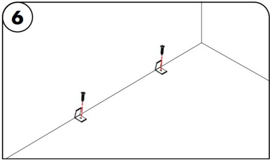
6.1 Screw mounting brackets into previously made markings from step 1, then clip the extrusion on to the mounting brackets.
