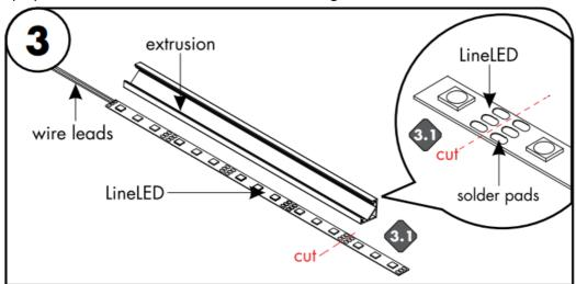
**Note:** Extrusion are not waterproof. If it is going to be installed facing up and in a wet location, drainage holes should be drilled along the inner corner of the extrusion every 12". Drill 1/16" to 1/8" diameters holes before installing LED strip
