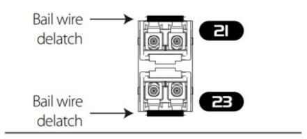
3. Open the bail wire to disengage and remove the mini-GBIC transceiver.
