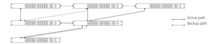
To create a redundant path with RLinkX, simply connect a minimum of two links between two GigaCore switches. The blue RLinkX LEDs of the connected ports will turn on, indicating the redundancy is active and available. If your port's RLinkX LED turn off, you have lost one of your redundant paths.
