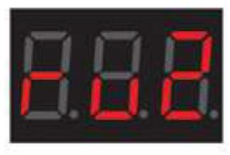
• B. Set DMX Decoder Address 2 If the controller is set to DMX Decoder mode r U you need to set the OMX address by holding any one of the buttons until display flashes, then click the button to set address, under the digit you wish to change.
