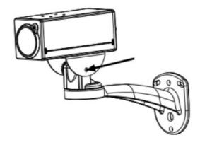
1. **Wall-mounted frame:** The camera is installed on the wall, using Lumens VC-WM11 (optional) wall-mounted frame
