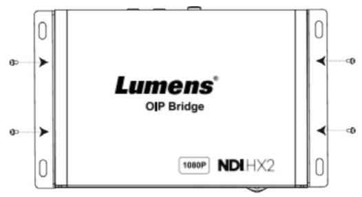
2. Install the metal plate and OIP-N60D under the table according to the spatial area
