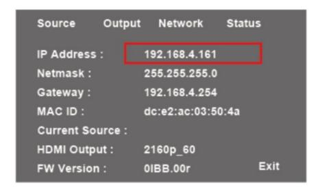
3.2 Open the browser and input the IP address, e.g. 192.168.4.161, to access the login interface.
