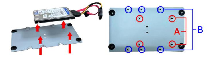
4.5 Lock the hard drive mounting plate in place and insert the connection cable.
