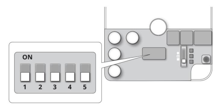
Set the baud rate, parity, and stop-bit configuration on the DIP switch to match the configuration of the connected Modbus device. The possible combinations can be found in the table to the right.
