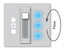
2. All powered W-Modbus Nodes within range will now connect to the Gateway. This process takes a few minutes. Nodes further away will connect to a closer W- W-Modbus Node if the Gateway is out of reach. When a Node is connected it will be indicated by a synchronous green blink on all three LEDs.
