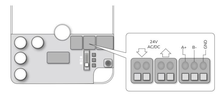
The W-Modbus units have 24 VAC/VDC power in/out connections and connections for Modbus RTU communication via RS485.
