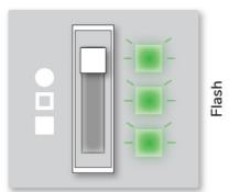
3. Check that all Nodes installed are indicating connection, and then set the 3 pole switch to the bottom position on the W-Modbus Gateway. Now the entire network will reboot into secure mode and be ready for operation. From now on the LEDs will indicate status in accordance with the system status section.
