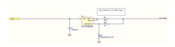
A more advanced PSU design can be achieved using the above circuit, which allow for more precise control over guaranteed PSU current while keeping the max current fairly close to the guaranteed.
