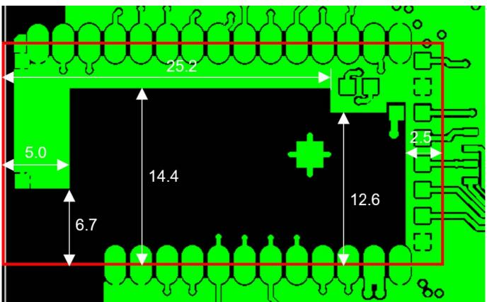
Guidelines for optimal performance for the internal antenna
