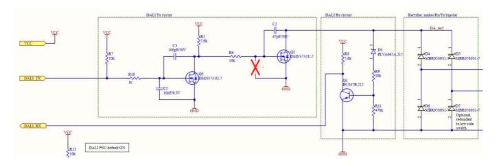
A DALI interface circuit to connect the W-DALI module to a DALI bus can be constructed as in the design above.
