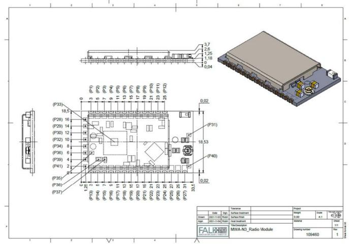
All dimensions in mm. The W-DALI OEM module is implemented on the LumenRadio MWA-N3 radio module. Mechanical design files in .stp and .dxf format is available for download at the LumenRadio online support page.
