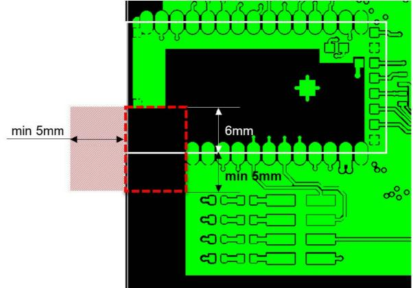
The keep-out area extends from the module PCB surface in the vertical directions as well. Note that the carrier board thickness can be included i the total distance below the module, so that given a 1.6mm carrier board, its standoff shall be minimum 3.4mm.
