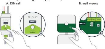
A – Move the switch to "COMM" or B – Move the switch to "  $\blacksquare$  ".
