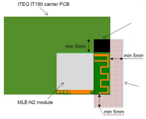
Black Area is a carrier board clearance area. No components or traces/GND planes are allowed in this area. This area should be min 5mm wide from the board edge of MLE-N2 to the opposite board edge. Please note the orientation of the antenna and MLE-N2. Red diagonal striped area is a keep out area "air gap" from any solid objects or carrier board PCB material.
