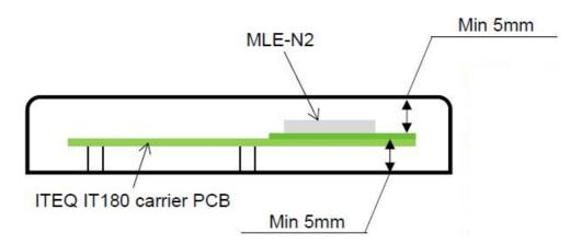
Min 5mm to solid objects under and above MLE-N2 antenna area. Note that carrier board thickness can be included in the total distance to solid objects under the antenna. I.e. for a 1.6mm carrier board standoffs needs to be min 3.4mm
