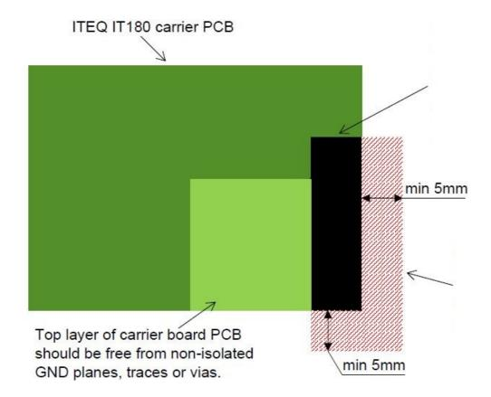
Black Area is a carrier board clearance area. No components or traces/GND planes are allowed in this area. This area should be min 5mm wide from the board edge of MLE-N2 to the opposite board edge. Red diagonal striped area is a keep out area "air gap" from any solid objects or carrier board PCB material.
