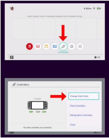
Once on the pairing screen pictured, hold down the SYNC button on the controller for at least three seconds. The player LEDS will cycle from left to right to indicate the controller is in pairing mode.
