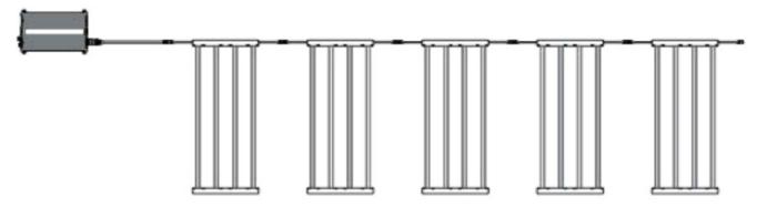
For alternative light plans and greater flexibility, extension connecting cables are available to purchase separately. Example of a vertical connection plan with extension connecting cables:
