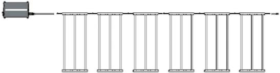
For alternative light plans and greater flexibility, extension connecting cables are available to purchase separately. Example of vertical connection plan with extension connecting cables:
