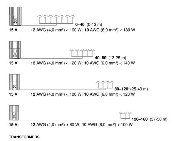
**Single transformer:** When using one transformer, center the transformer on the wattage load. Minimize all cable runs to reduce voltage drop.
