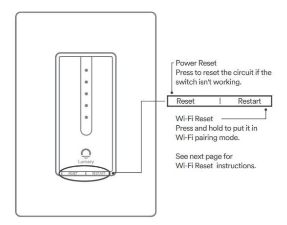
How do I reset TAP and what does the blinking light mean? Reset TAP by pressing and holding the Wi-Fi Reset (Restart ) button for 3 seconds until the indicator begins to rapidly flash. The Wi-Fi Reset button is located on the bottom right side of the switch (not the swashplate) labeled "Restart".
