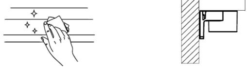
3. Please use the 3M glue in the accessory bag, peel off the 3M surface layer on the back, and stick it on the back or top of the permanent down light according to your needs. It is recommended to align the light tightly with the edge of the fixture at right angles to the wall, and then press it firmly to stick it firmly. It can also be installed and fixed with screws
