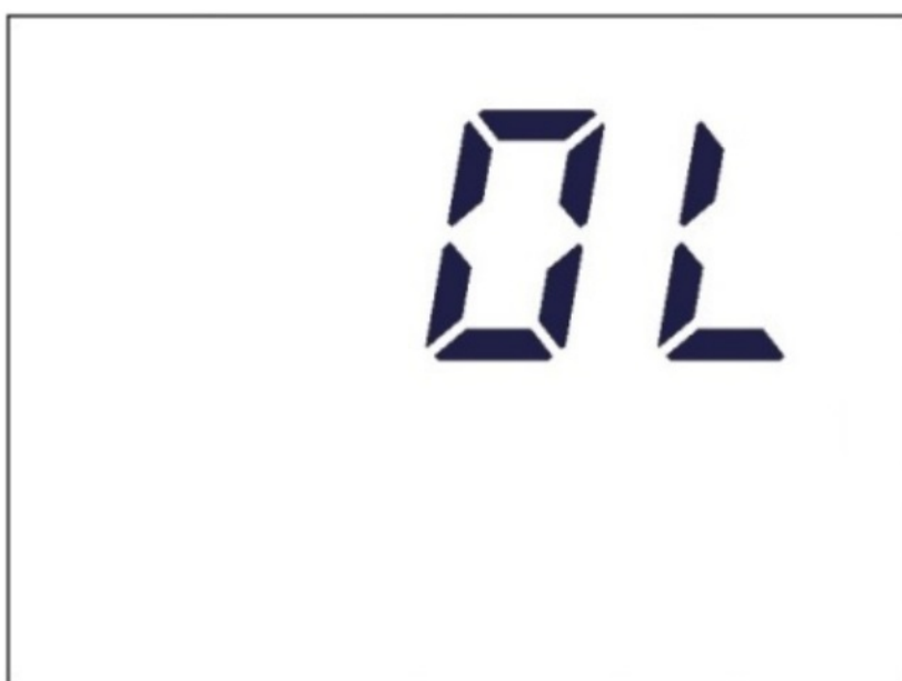
Figure 2.7: Detector Overload Alarm (Display Will Flash)
