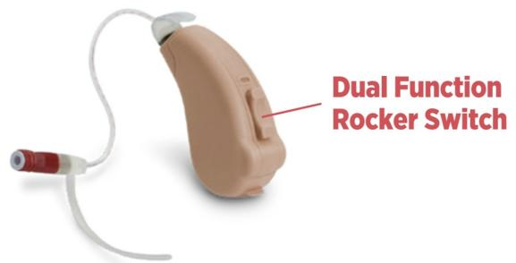
Once the battery door is completely shut, you will hear the unit turn on. To adjust the volume either higher or lower use the Dual Function Rocker Switch. You will press either up or down and quickly release the rocker switch (do not hold down). You will hear double tones indicating the volume has been adjusted. If you do not hear the tones, this indicates you have reached the maximum or minimum hearing volume level. Always ensure the volume is at a comfortable listening level.
