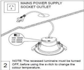
NOTE: The recessed luminaire must be turned off before using the switch to change the colour temperature.
