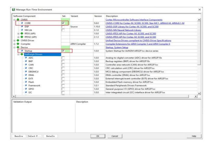
Add peripheral library support, for example, add GPIO library, check the GPIO component after you can see the following will prompt the lack of other components, according to the prompt to check, you can also check all.
