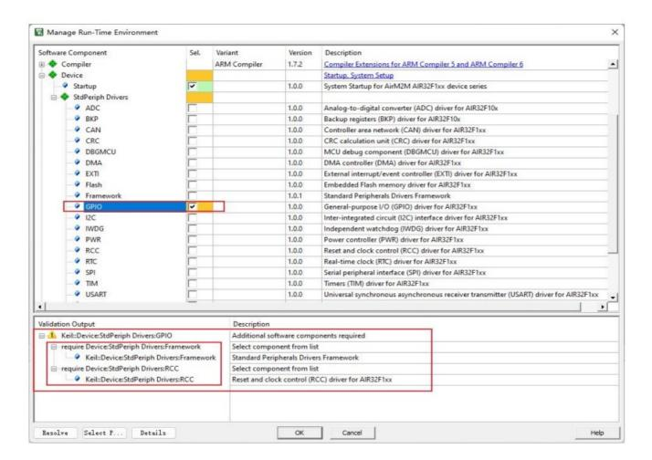
After checking the missing dependencies according to the prompt, the prompt is removed and the project is created by clicking OK.
