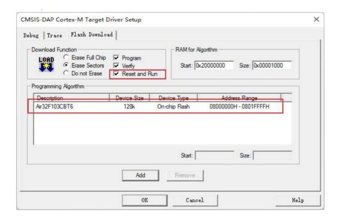
After the configuration is completed, you can click on the burn button to download and burn the code to the device directly.
