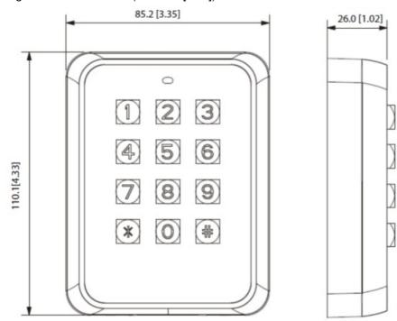
• Figure 1-2 Dimensions of the LXK101-KD (mm [inch])
