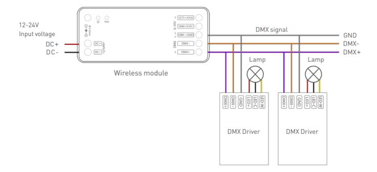
Covert Bluetooth signal to DMX signal, and connect to DMX dimmable drivers to control DIM/CT/RGB/RGBW/RGBWY.
