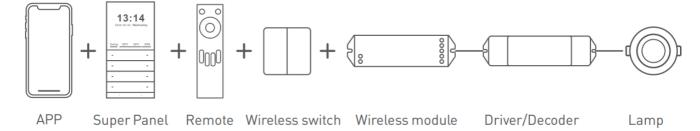
4. Link up the intelligent touch panel with the module by App to control the lamp simultaneously by App, Super Panel and touch panel.
