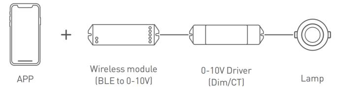
2. Link up the wireless module(After BLE to DMX) by App to achieve fast dimming control.
