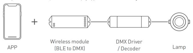
3. Link up the Super Panel with the wireless module by App to realize visual control + remote control of traditional panels.
