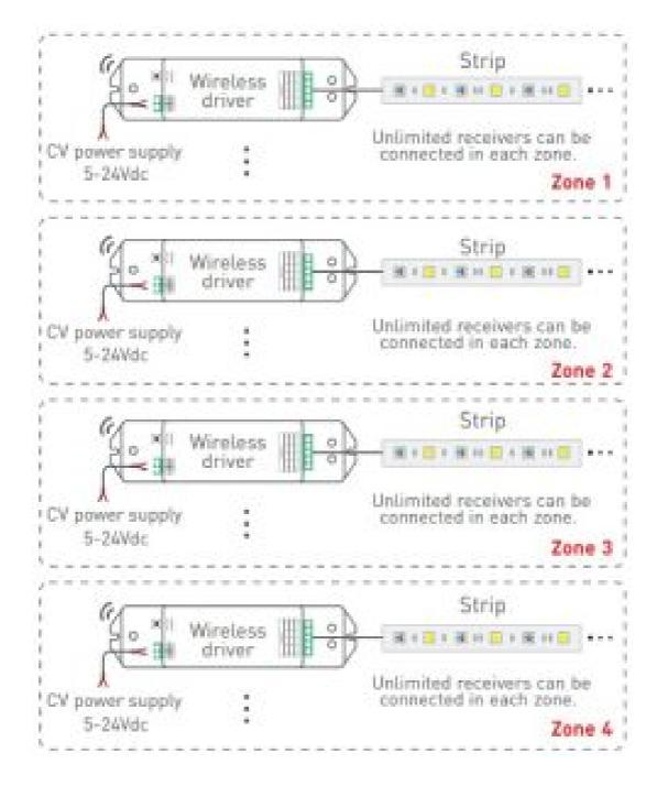
Multiple wireless receivers (F4-3A/ F4-5A/F4-DMX-5A/F5-DMX-4A) can be matched with EX series touch panel within effective distance.
