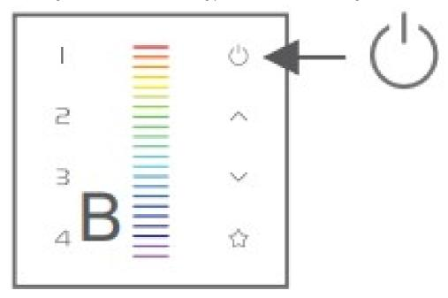
2. Touch the matching zone key on A within 15s, when indicator lights of B stop flicking, match successfully.
